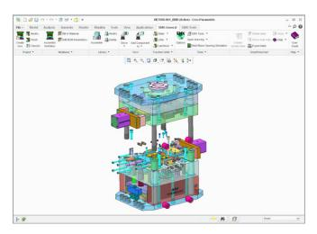
An exploded moldbase in Creo Expert Moldbase Extension.
